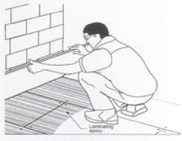
Figure 15 Lay 4.5mm sheets across bottom sheets
